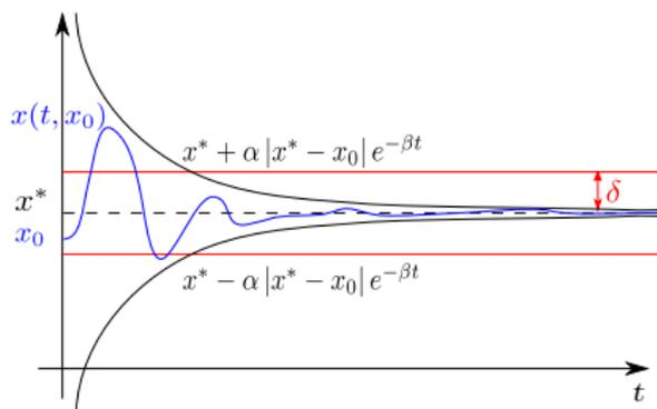
$$\|x_0 - x^*\| \leq \delta \Rightarrow \|x(t) - x^*\| \leq \alpha \|x_0 - x^*\| e^{-\beta t}, \forall t \geq t_0.$$
